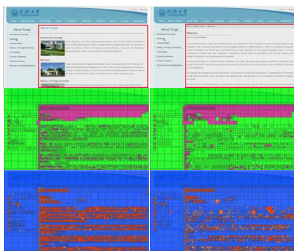
Figure 11. SCC-HEVC Transcoding Analysis of "WebBrowsing" (QP=22) Top Left: 8 th Frame; Top Right: 9 th Frame; Mid Left: Anchor Transcoding Mode and Partition Decisions; Mid Right: Proposed Transcoding Mode and Partition Decisions; Bottom Left: Anchor Transcoding Bit-Allocation Heatmap. Bottom Right: Proposed Transcoding Bit-Allocation Heatmap. Red box: Intra-coded blocks; Green box: Inter-coded blocks; Blue box: low-bit blocks; Orange box: high-bit blocks with color depth indicating bit-consumption level.
